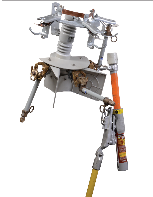
Figure 11. Detaching the Loadbuster tool from Three-Shot Fuse Cutout.
