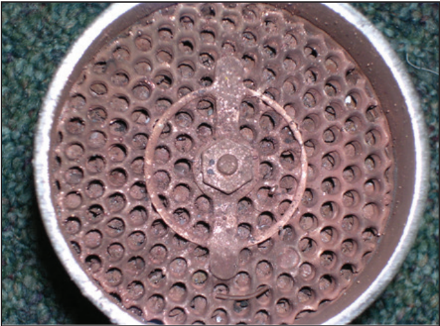
Figure 8. Silencer after one operation at full fault current.
