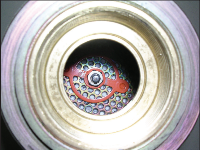
Figure 7. Silencer with a red INTERNAL WEAR indicator.
