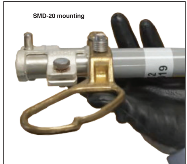
Figure 5. An SMD-20 Power Fuse upper ferrule without a bronze spacing washer.
