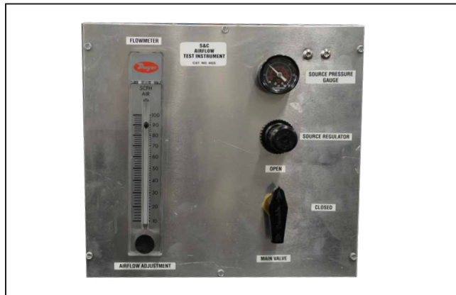
Figure 4. Adjust the airflow adjustment valve to obtain an airflow of 90 SCFH.
