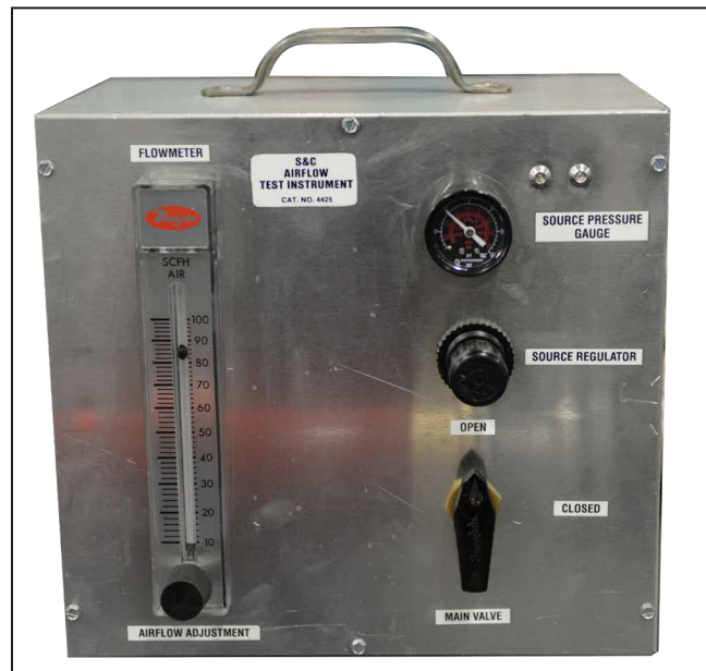
Figure 8. Read and record the airflow value on the flowmeter scale.
