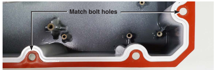
Figure 4. Match gasket holes with bolt holes.
