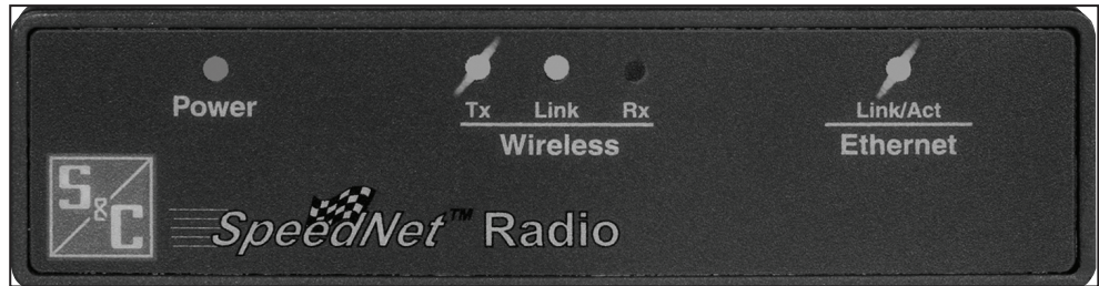
Figure 9. Wireless - Link LED indicator is lit, and Wireless - Tx and Ethernet Link/Act LEDs are flashing.
