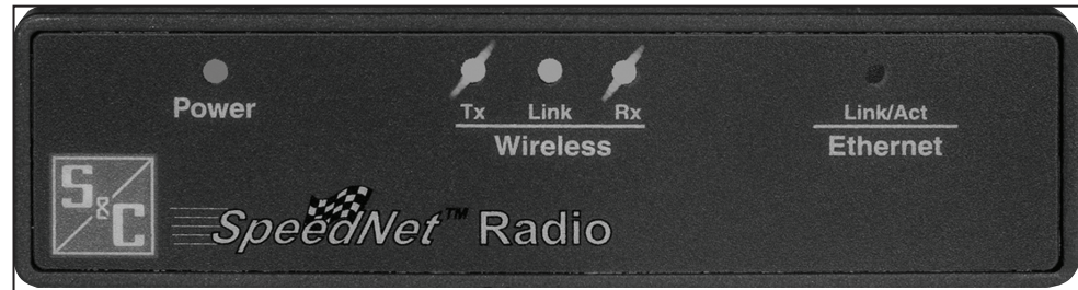
Figure 11. Wireless - Link LED indicator is lit, Tx and Rx LED indicator are flashing.
