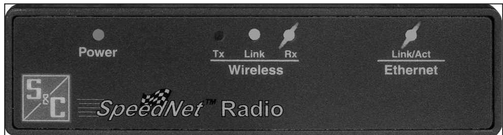
Figure 10. Wireless - Link, LED indicator is lit, and Wireless - Rx and Ethernet Link/Act LED indicator are flashing.
