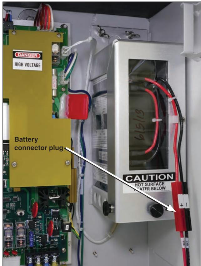
Figure 5. The battery connector.
