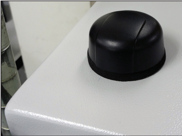
Figure 4. Exterior view of the installed GPS antenna.
