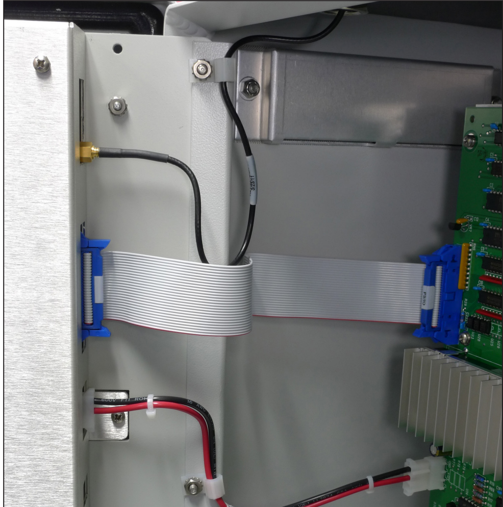
Figure 8. The GPS antenna connection is inside the top port on the hinge side of the processor-board shield.
