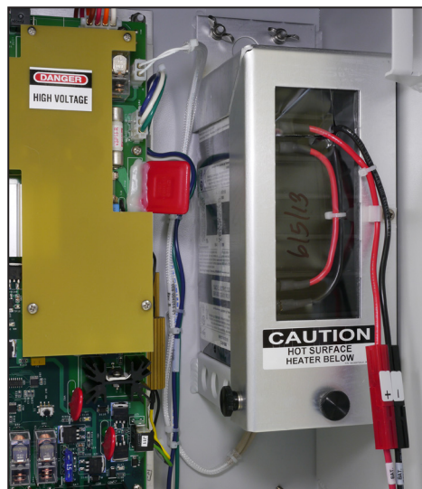
Figure 21. Battery and bracket on the right, inside the switch control enclosure.
