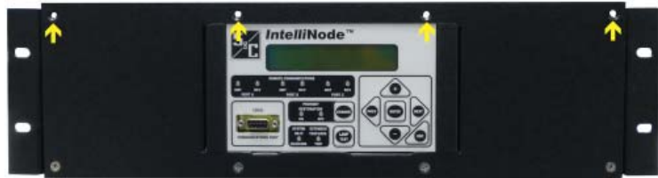
Figure 3. Top plate attachment screw locations on the front panel.
