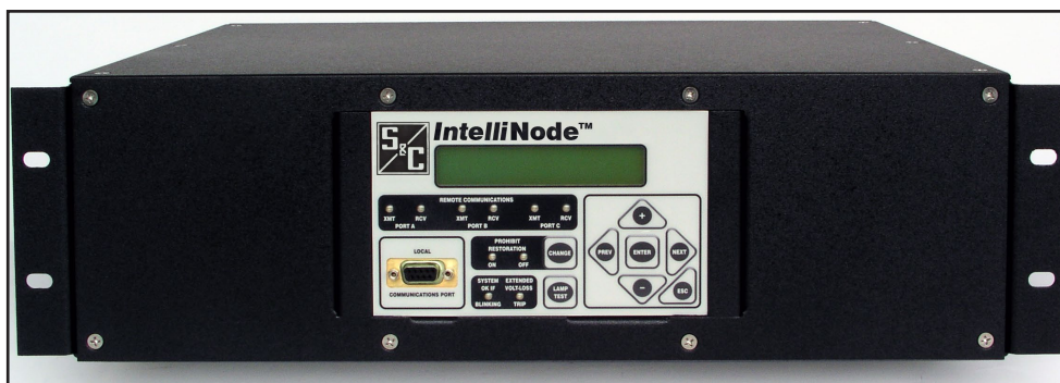
Figure 2. A rack-mounted IntelliNode Interface Module.
