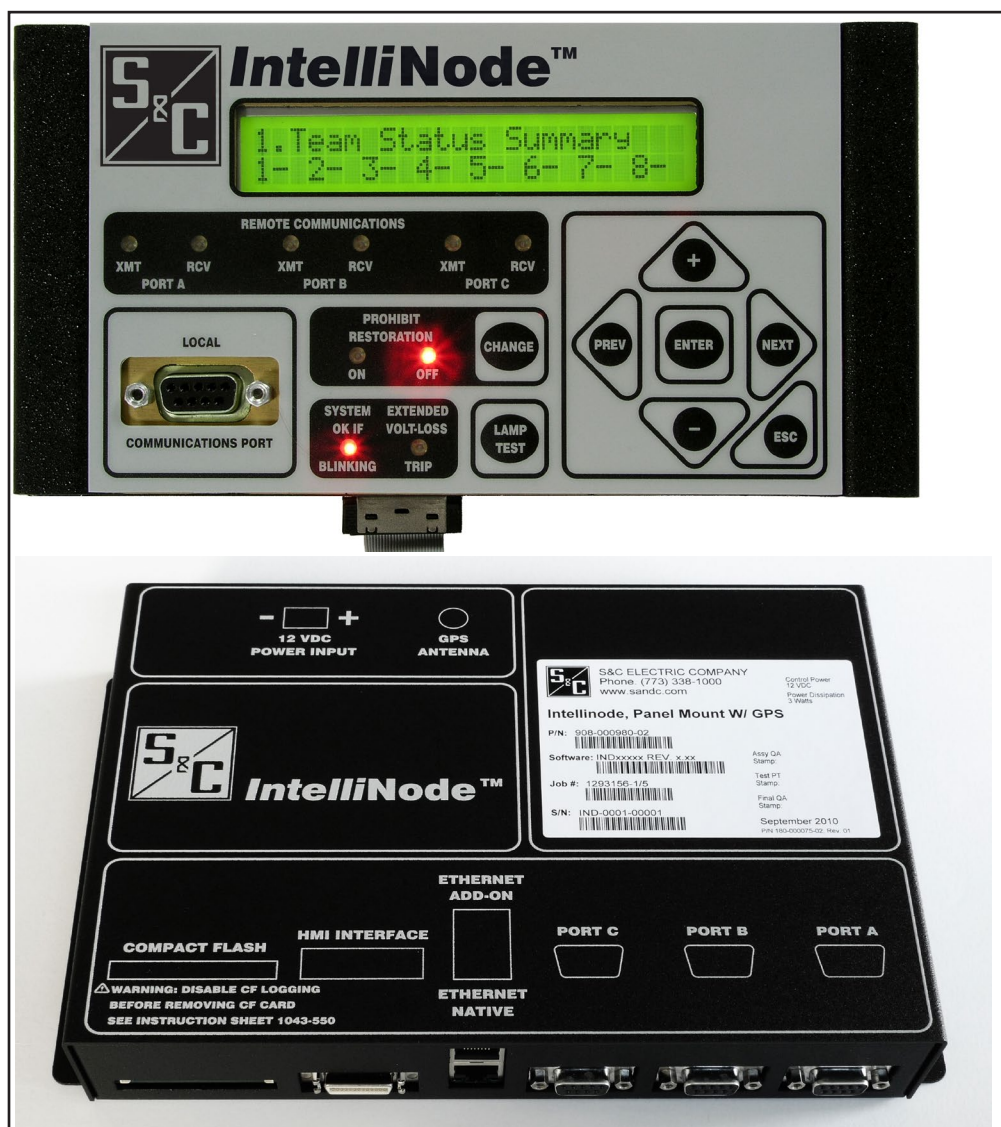
Figure 1. The remote faceplate and main chassis of the panel-mounted IntelliNode Interface Module.
