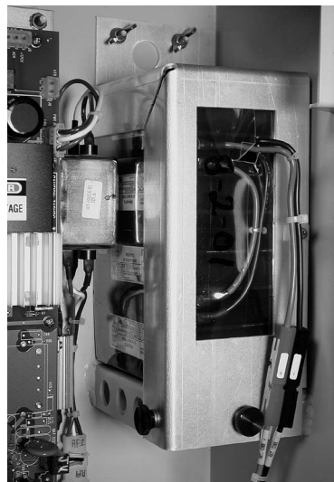
Figure 12. Battery and bracket are on the right, inside the switch control enclosure.
