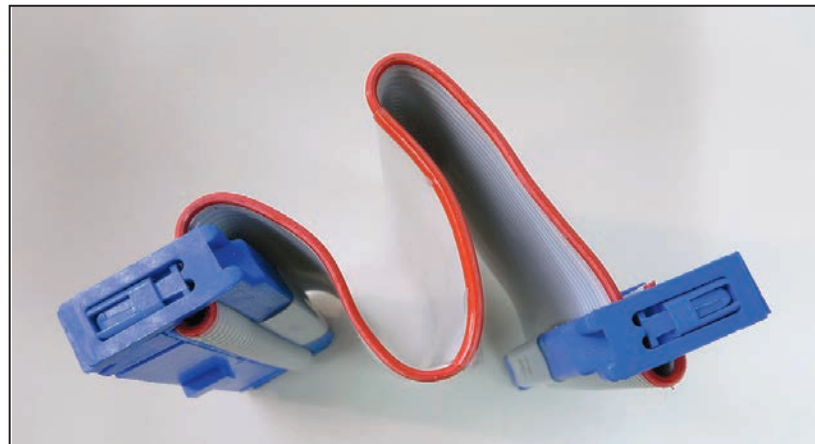
Figure 26. Harness to connect front panel, bent so it will not be crimped.
