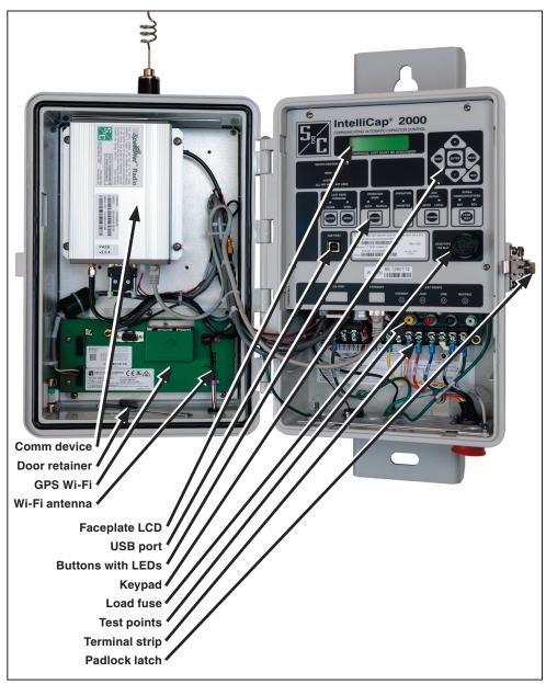
Figure 2. Interior of the IntelliCap 2000 control.
