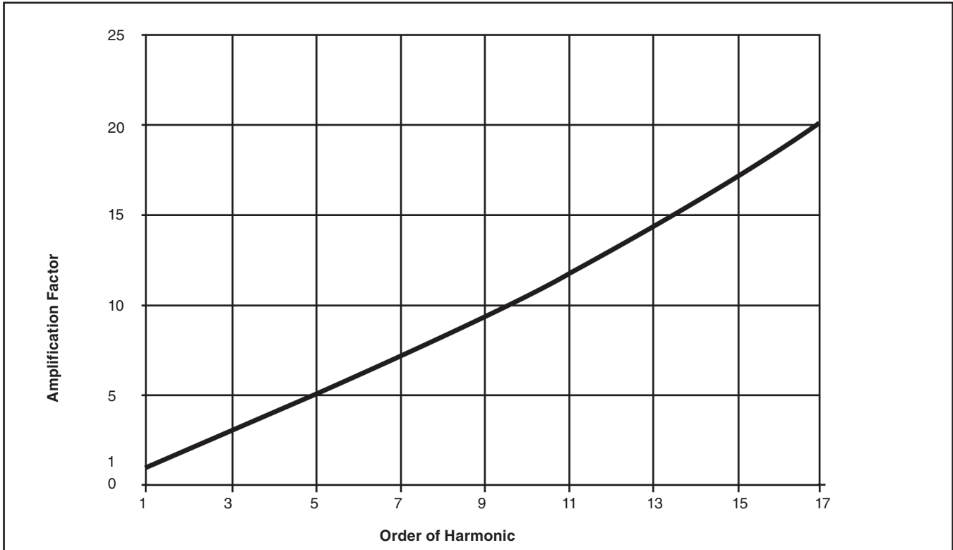
Figure 4. Amplification factor versus the order of harmonic for a 5-Vac nominal voltage sensing output at 25°C (77°F). Applicable to S&C Voltage Sensors of all ratings.
