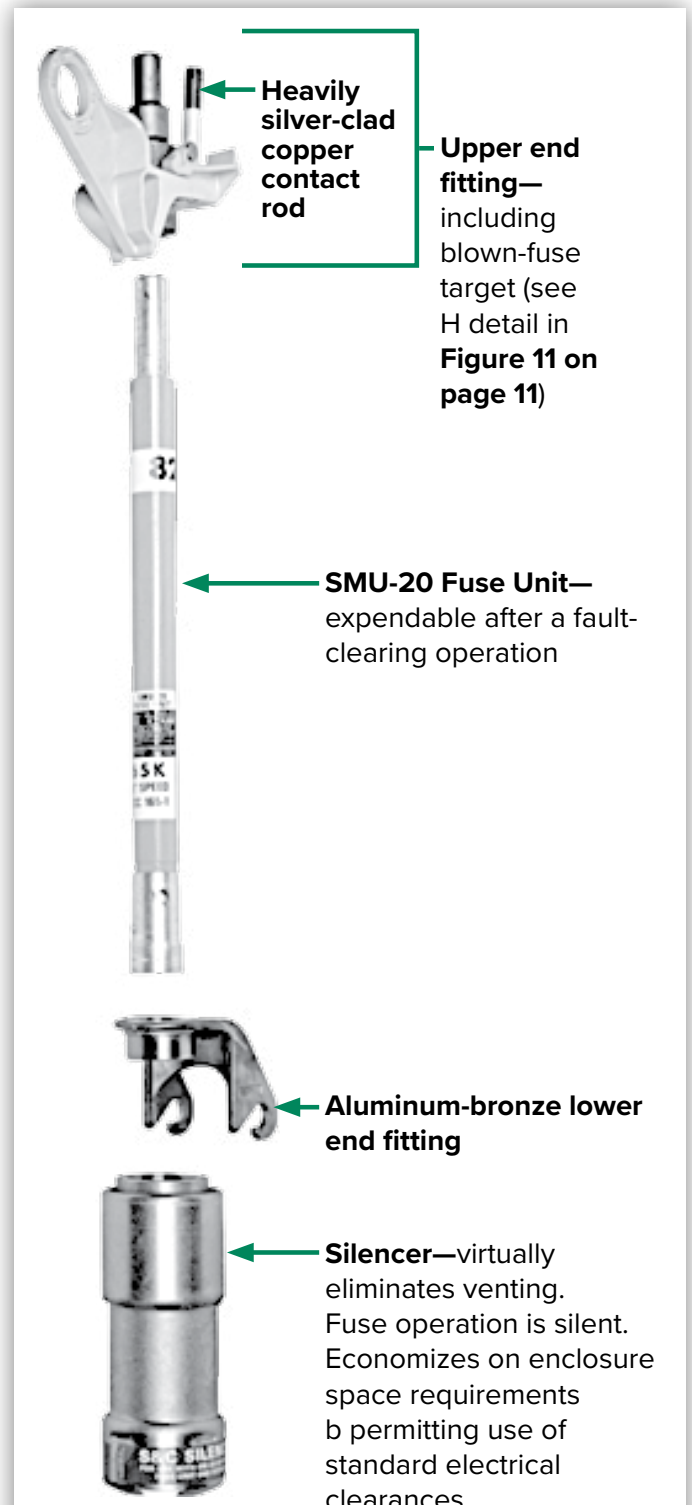
FIGURE 7. SMU-20 fuse unit and end fitting assembly.
