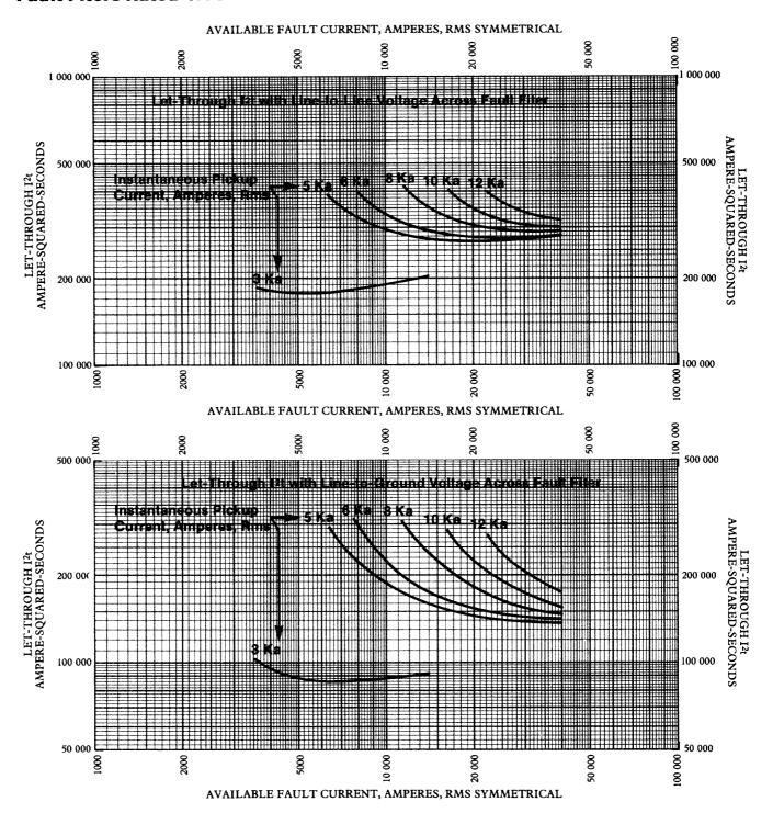
NOTE: The let-through I<sup>2</sup>t curves shown are based on the full spectrum of circuit X/R ratios from 3 through 20, and all degrees of asymmetry.
