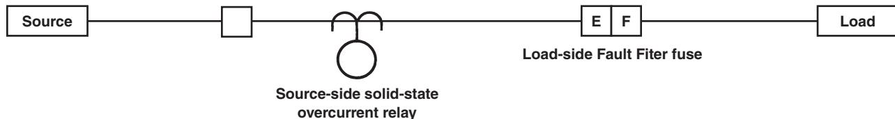
The selection tables presented in this information bulletin feature minimum pickup currents and time-dial settings for source-side solid-state overcurrent relays selected to provide complete coordination with load-side inverse-curve-type Fault Fiter Electronic Power Fuses. These curves also can be found in Coordinaide™—The S&C Protection & Coordination Assistant.
