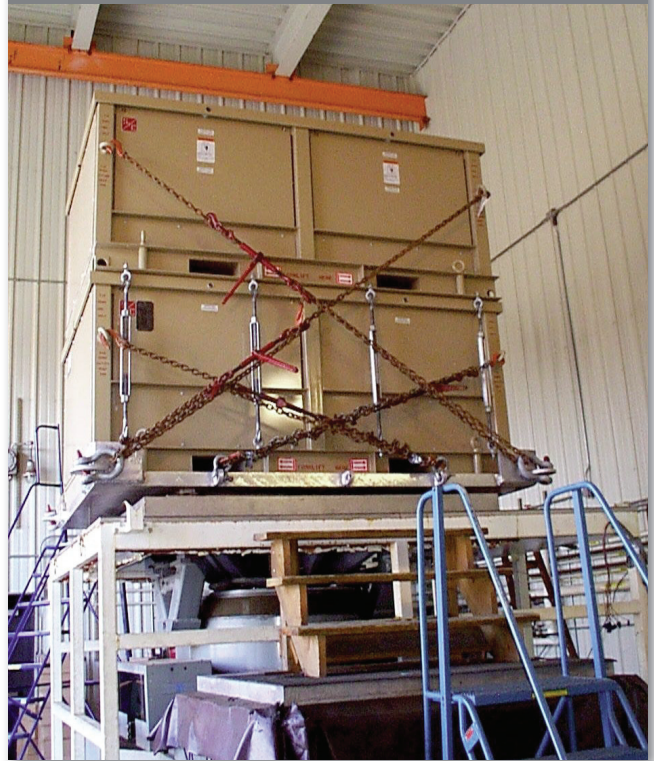
Stacked Vista switchgear units undergo the military's arduous shaker table vibration test.
