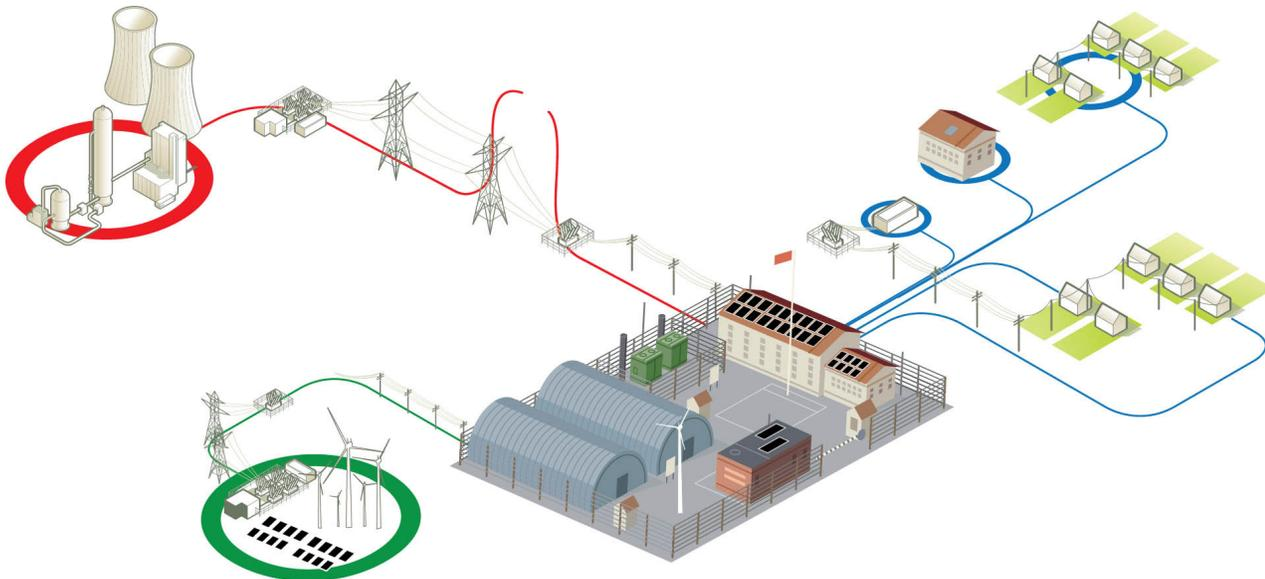
Energy storage systems can provide a back-up power supply in the event loads are disconnected from the central power grid. They can also make renewable power generation a practical power supply for islanded loads.
