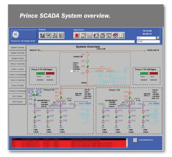
A supervisory control and data acquisition and fiberoptic communication system provides operation and maintenance personnel with real-time information on the state of the wind farm equipment, as well as realtime control to meet operational needs. The system also provides data access to the transmission system operators the Ontario System Control Center.
