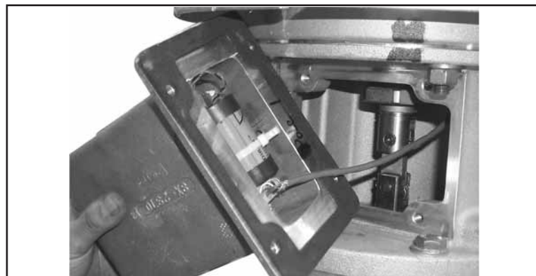
Figure 6. Reattach the transmitter to the transition box after making the battery and sensor cable connections.
