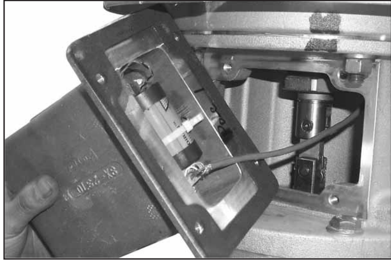
Figure 25. Reattach transmitter to transition box. Make sure that the black antenna panel is facing the ground.
