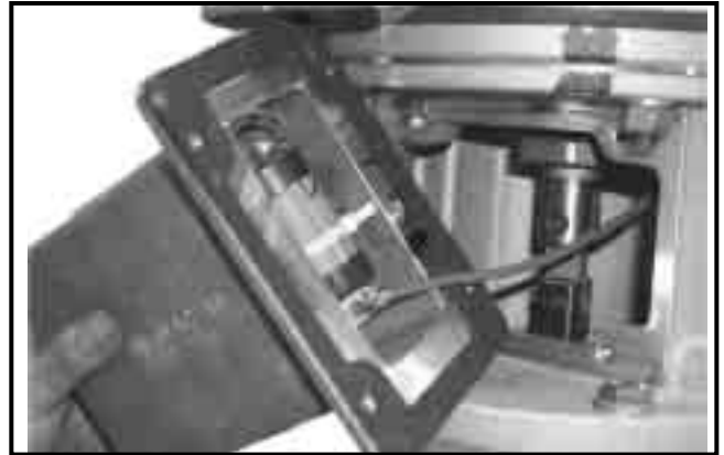
Figure 19. Reattach the transmitter to the transition box after making the battery and sensor cable connections.
