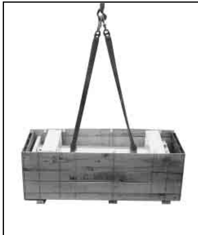
Figure 6. Removing replacement interrupter from shipping crate.
